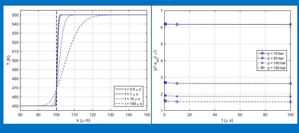
Left – temperature profile at different times at 150 bar.
